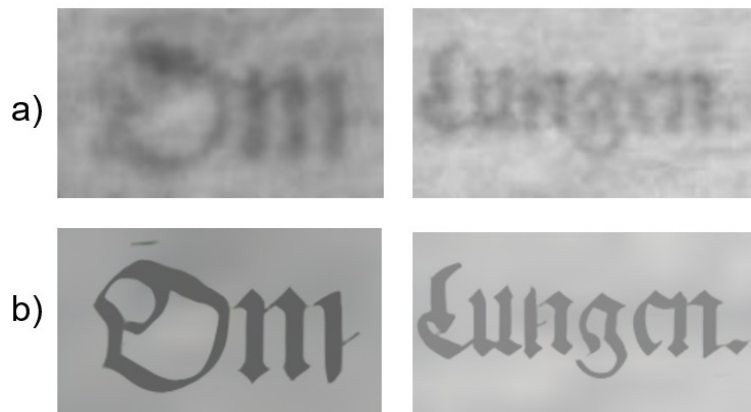
Figure 8: Qualitative performance of the model on degraded text images "Om" and "Lungen" extracted from the fragment on Herlufsholm 24.1. The figure shows a) the LR inputs and b) the SR outputs.
